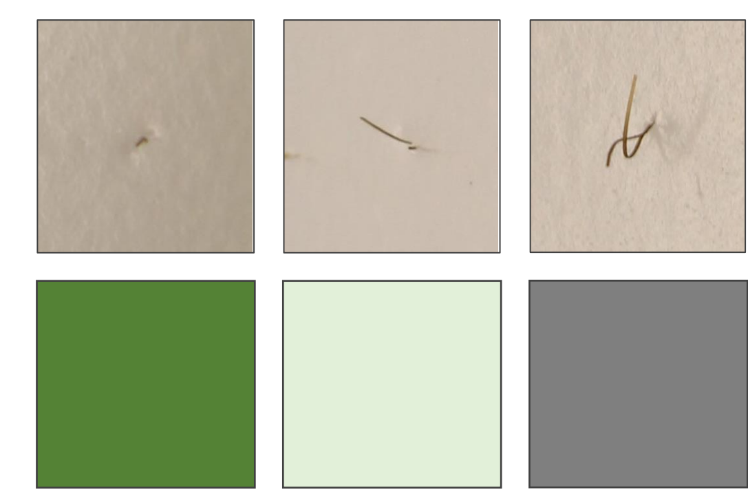
Fiber removal grading scale (left to right) 2 fibers, 1 fiber, 0 fibers removed
