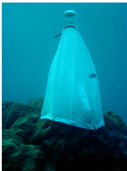
FIGURE 2.3 A mesh tent used for in situ collection of coral gametes during spawning events. SOURCE: Sharp et al., 2010.
