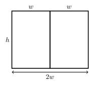
The objective function is the amount of fencing used (or perimeter of the figure), P = 4w + 3h. To express this function in terms of a single variable, we use the constraint given by the fact that the total area is 2,400 ft<sup>2</sup>. This gives 2wh = 2400, so  $h = \frac{1200}{w}$ . Therefore, the objective function in terms of the variable w is  $P(w) = 4w + \frac{3600}{w}$ .
