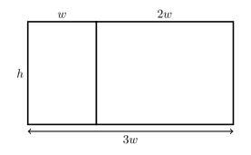
The objective function is the total area of both pens A = 3wh. To express this function in terms of a single variable, we use the constraint given by the fact that the amount of fencing is 360. This gives the equation 6w + 3h = 360, so h = 120 - 2w. Therefore, the objective function in terms of the variable w is  $A(w) = 3w(120 - 2w) = 360w - 6w^2$ .
