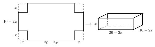
The objective function is the volume of the box  $V(x) = x(10 - 2x)(20 - 2x) = 4(x^3 - 15x^2 + 50x)$ . To find the interval of interest, observe that all lengths must be postive, so we need  $x \ge 0$ ,  $10 - 2x \ge 0$  and  $20 - 2x \ge 0$ . This gives the interval [0,5]. We now use calculus to find the absolute maximum of  $V(x) = 4(x^3 - 15x^2 + 50x)$  on [0,5].
