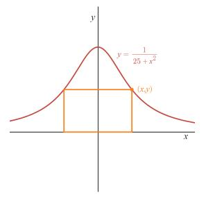
The rectangle has base 2x and height y. The objective function is the area A = 2xy. The constraint is given by the fact that (x, y) is a point on the graph, which gives the equation  $y = \frac{1}{25+x^2}$ . Therefore, the objective function in terms of the variable x only is  $A = \frac{2x}{25+x^2}$ .
