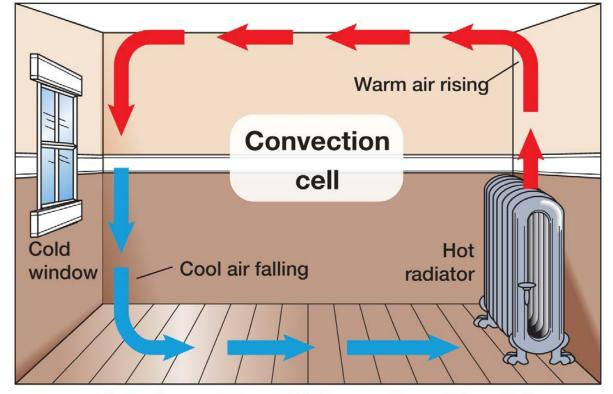
A circular-moving loop of air (a **convection cell**) is created in this room by warm air rising and cool air sinking.
