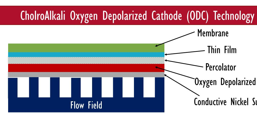
ODC technology is state-of-the-art in the ChlorAlkali industry. ODC electrodes consist of electrocatalyst that thermodynamically favor the production of NaOH and Cl<sub>2</sub>. The large scale implementation of the ODC electrode calls for an electrolyzer architecture that would enable maximum catalyst activity while minimizing cell overpotential.
