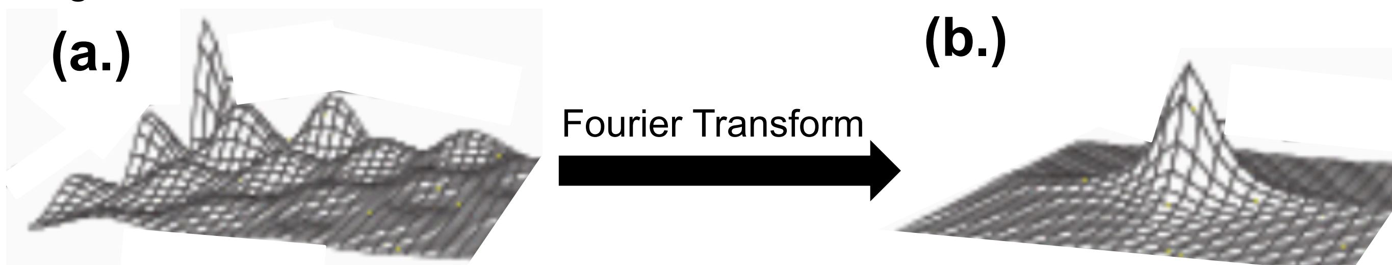
Figure 4. Demonstration of how stacked 1D FIDs can create a 2D FID and be used to generate multidimensional spectra, modified from 2. Alternating conditions slightly between collection cycles allows for the collection of an indirect dimension. This can be used to show the resonance between atoms. a. Array of 1D FIDs lined up to make a 2D FID. b. Spectrum after mathematical transformation.
