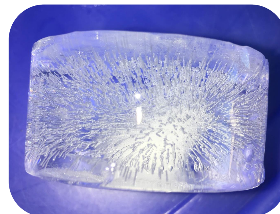
Figure 1: Image of an ice cube frozen in a standard freezer with distilled water.
