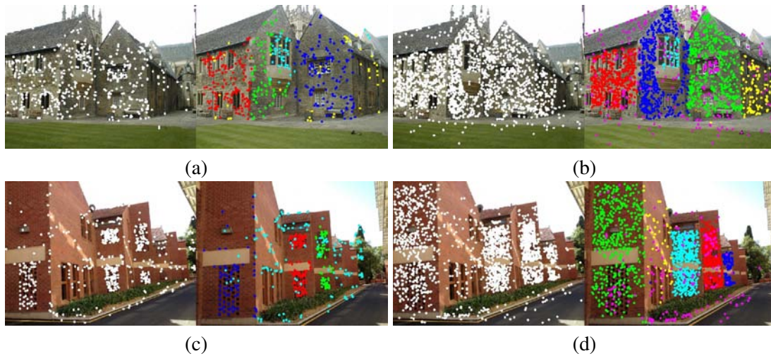
Figure 4.8: Homography estimation. (a) Merton College with 536 point pairs. Four inlier and one outlier structures. (b) Merton College with 1982 point pairs. Five inlier and one outlier structures. (c) Unionhouse with 619 point pairs. Three inliers and one outlier structures. (d) Unionhouse with 2084 point pairs. Five inliers and one outlier structures.
