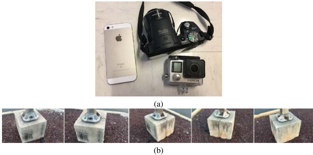
Figure 5.1: Capture of a 2D image sequence. (a) The three cameras used to capture different videos. (b) Five 2D frames extracted from the video used in the example.
