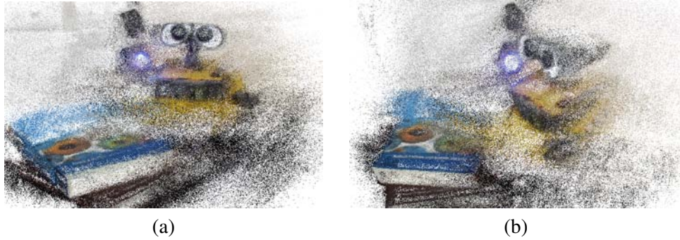
Figure 7.1: Heteroscedastic noise in the 3D triangulation. (a) Error is low in the front view. (b) Stronger error is observed along the depth direction.
