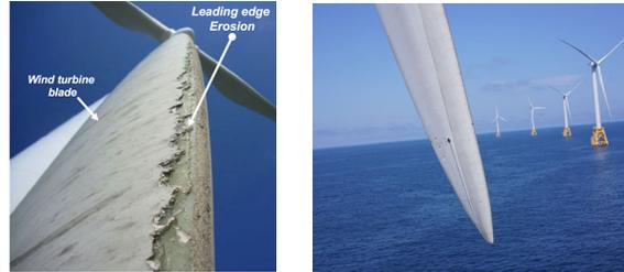
Leading edge erosion is often caused by raindrops, hailstones or other particles impacting the leading edge of the blade. In turn, this causes the material to be removed off the surface of the blade, leaving a rough profile that degrades the performance of the blade over time.
