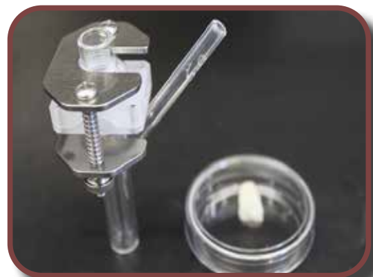
Figure 7: Franz diffusion cell with nail adapters
