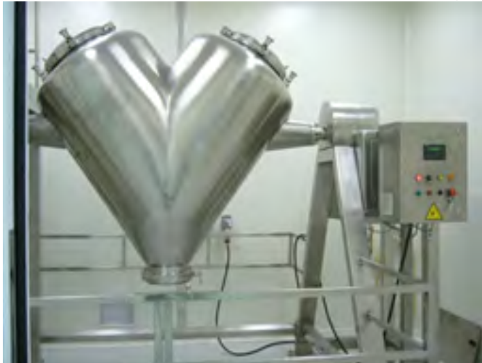
Fig. 1. Blenders used for this work: (a) 7.5-L V-blender and; (b) 7.5-L conical bin-blender. M. Lemieux et al., Chemical Engineering Science 62 (2007) 1783-1802.
