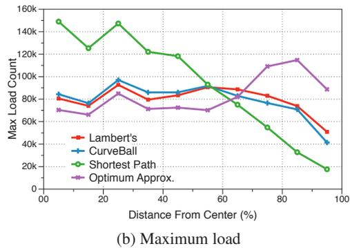
**Figure 4.** Histogram of (a) average load and (b) maximum load as a function of distance from the center. The network has 1500 nodes on a perturbed grid.
