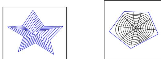
(b) Contoured star-shaped polygon using shrinking boundary method (c) Contoured pentagon using conformal mapping method
