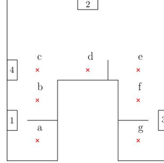
Fig. 2: Experiment testbed of covering targets using a camera network. There are 4 cameras (rectangles) with line-of-sight coverage and 7 point targets (represented by red crosses).
