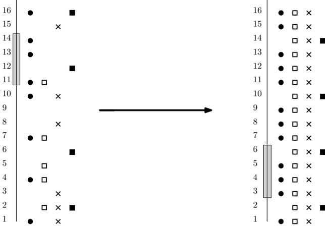
Fig. 3: Transforming a computable schedule to a periodic one. The example has  $T = 4$ . The disk, cross etc. represent different sensors, and their appearance represents the time slot they are scheduled. The interval  $[11, 14]$  corresponds to a target covered by a sensor shown as a empty box. The corresponding interval  $[3, 6]$  is also covered.
