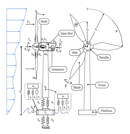
Considering more Degrees of Freedom allows to design advanced controllers for load alleviation
