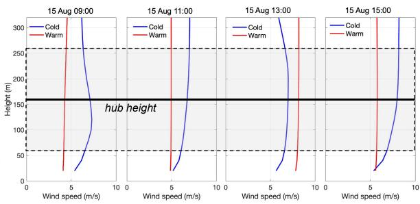
Power is proportional to cubed wind speed! Total energy over a two-day model (RU-WRF) run:
