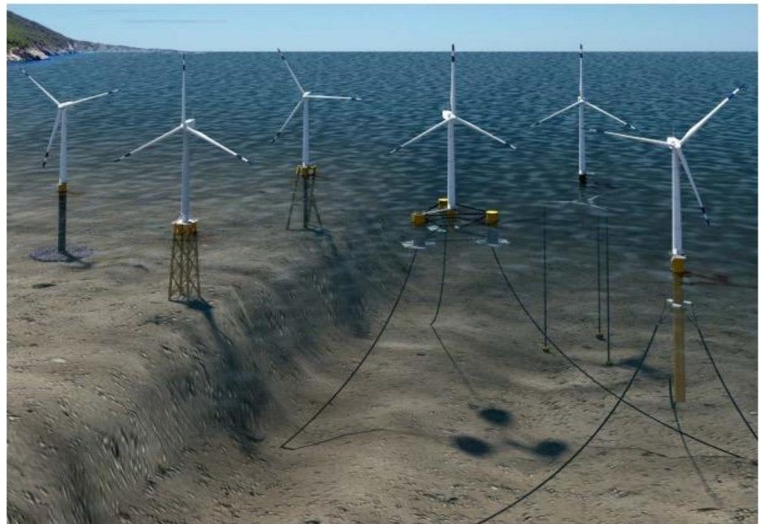
Figure 3.3. Six different offshore wind substructure types. The three on the far left are fixed-bottom substructures (monopile, jacket, and inward battered guide structure [also known as a twisted jacket]), and the three on the right are floating substructures (from left: semisubmersible, tension leg platform, and spar). Illustration by Josh Bauer, NREL.
